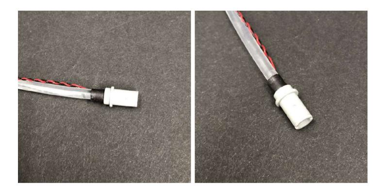
Connect the cool white light bar inside the vehicle via the technic pin ensuring the cable is on the bottom side of the bar.
