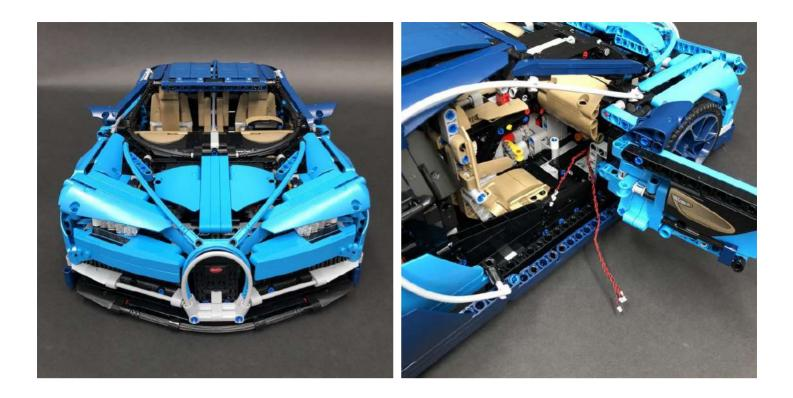
**8.)** Take a **12-Port Expansion Board** and connect all the cables from both headlights to it starting with those from the right headlight first.
