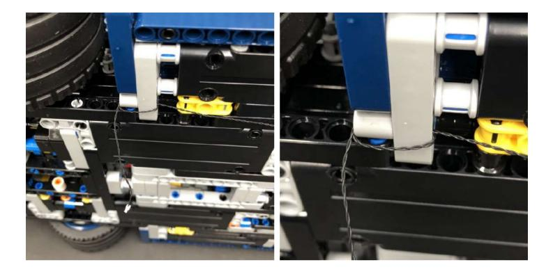
Connect the cable to the second 12-Port Expansion Board
