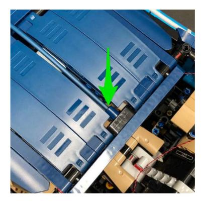
**11.)** Thread the Light Bar cable underneath the following technic piece and then connect it to a spare port on the 12-port expansion board.
